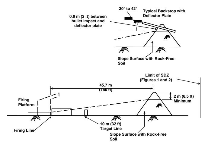
Figure 11. Machine Gun, 10-Meter Tube Range Typical Cross-Section
