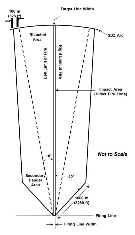
Figure 1. SDZ Configuration — Firing Line Width Equal to Target Line Width
