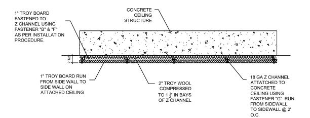
ATTACHED CEILING DETAIL (SIDE VIEW)
