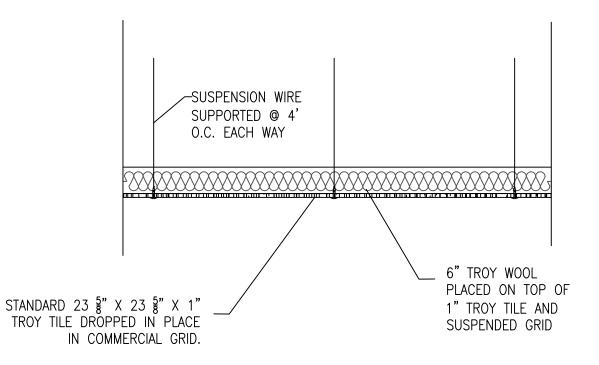
NOTE: COMMERCIAL 2'x2' TILE GRID (SUPPLIED BY OTHERS). GRID MUST BE SUPPORTED EVERY 4' IN EACH DIRECTION.
