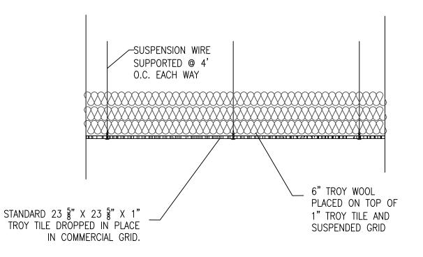
Standard Suspended Ceiling Install Procedure
