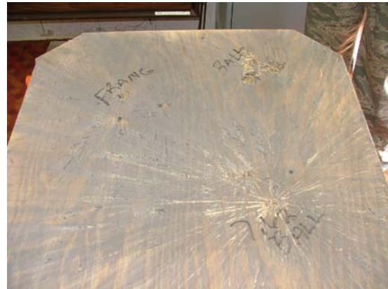
Figure 3.15. Rifle Impacts Rear Plywood
